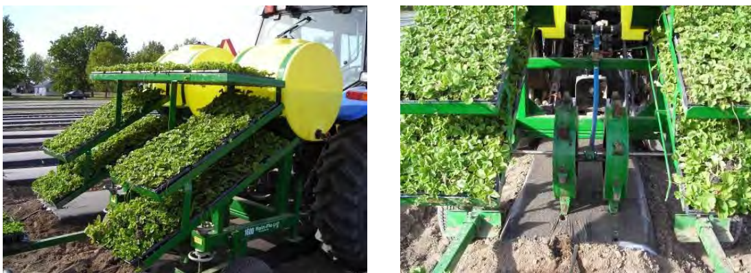
Figure 5. Strawberry plants can be mechanically transplanted on plastic mulch with a Rain-Flo™ Water Wheel Transplanter.
